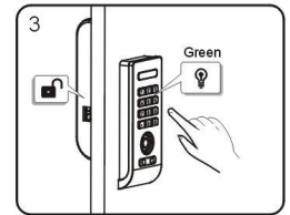
While the green LED light is flashing, press * and #, the green LED light will keep flashing
