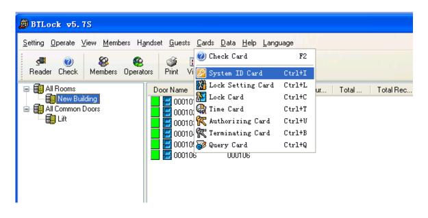
Step 3 Change the system password as you like. Put a Mifare S50 card on encoder, and then press the "Issue" button. After 1 beep, this card becomes to SID Card. Touch the SID to the front control panel of lift, then 1 beep with green light, done.
