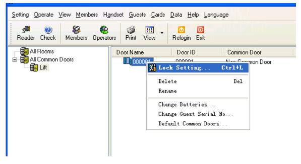
card becomes to Lock Setting Card. Touch the Lock Setting Card to the front control panel of lift., then 1 beep with green light, done.
