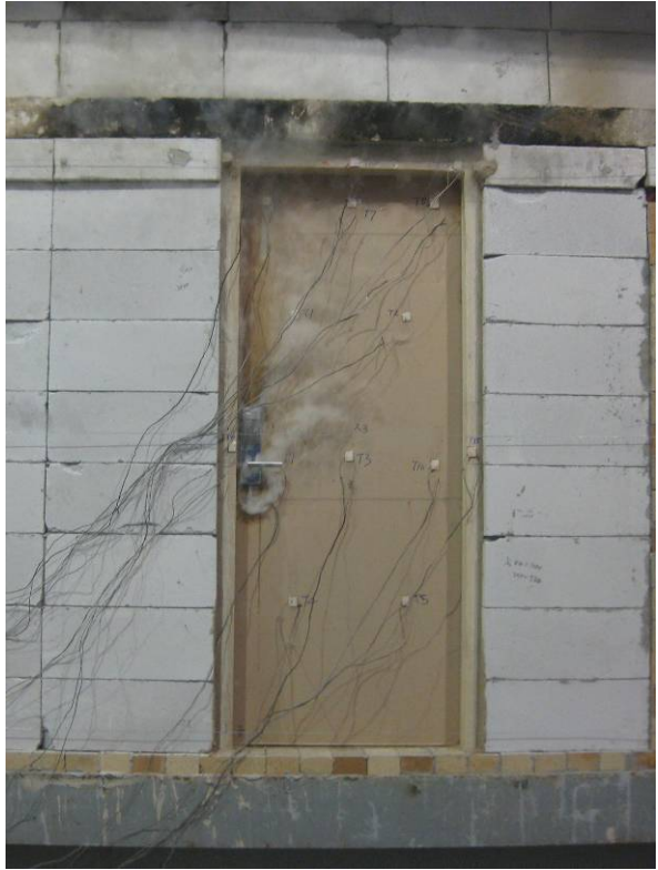
Fig. 4 – Unexposed Side after 9 Minutes
