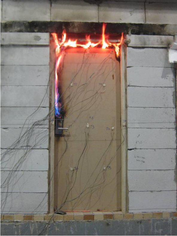
Fig. 7 – Unexposed Side after 55 Minutes
