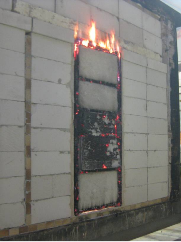
Fig. 8 - Exposed Side after 60 Minutes
