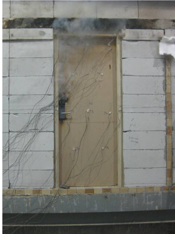
Fig. 5 – Unexposed Side after 25 Minutes
