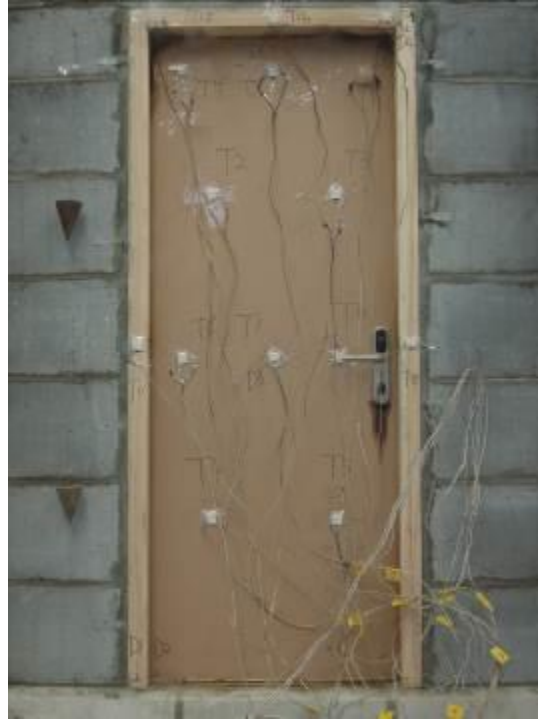
Fig. 9 – Unexposed Side after 60 Minutes
