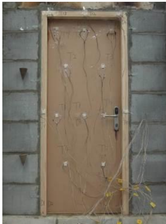
Fig. 6 – Unexposed Side after 30 Minutes
