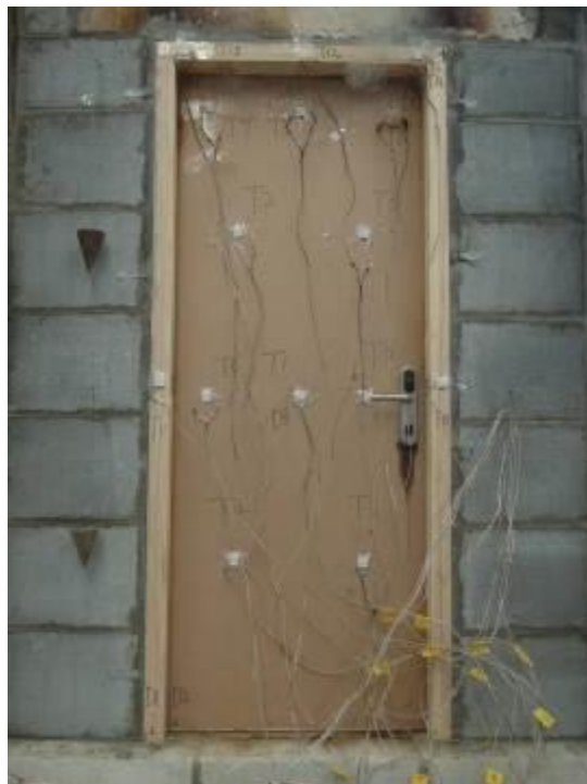
Fig. 8 – Unexposed Side after 50 Minutes
