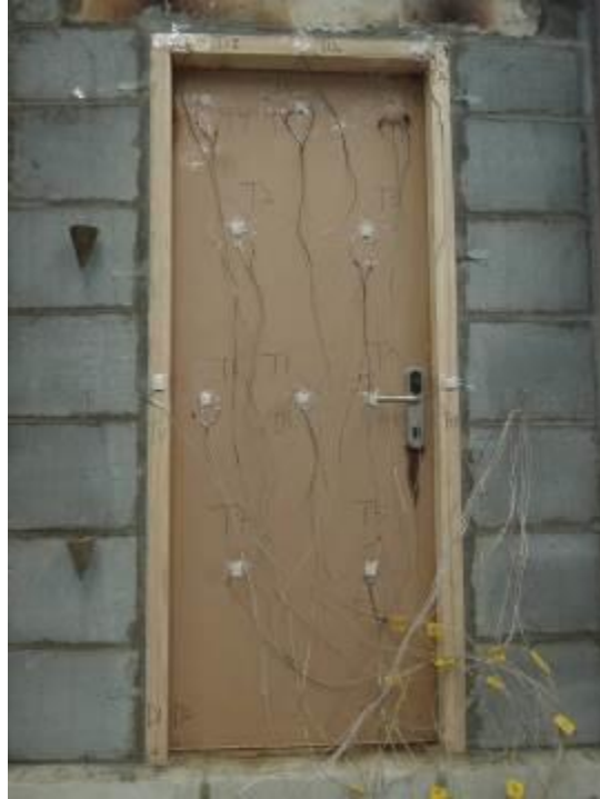
Fig. 7 – Unexposed Side after 39 Minutes
