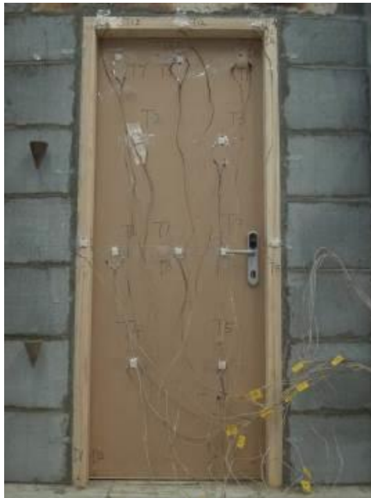
Fig. 2 – Unexposed Side Prior to the Fire Test
