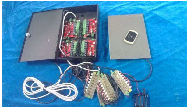
Testing Assembly View (32 LED lights simulated floor button indicator, and they are provided by the manufacturer)
