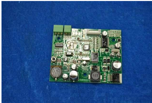
View of access control main board
