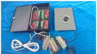
Testing Assembly View (32 LED lights simulated floor button indicator, and they are provided by the manufacturer)
